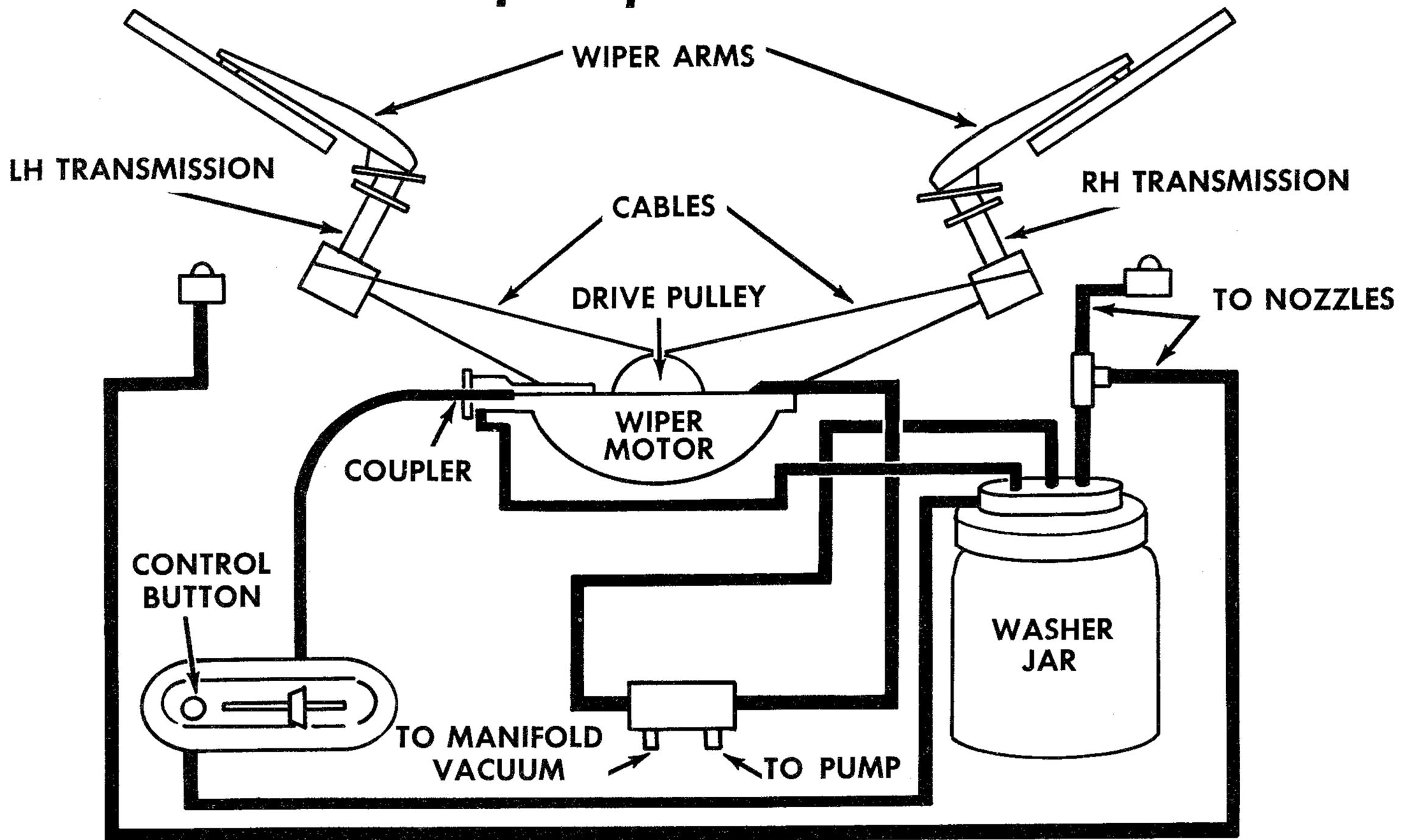
The windshield wiper also has mechanical controls
