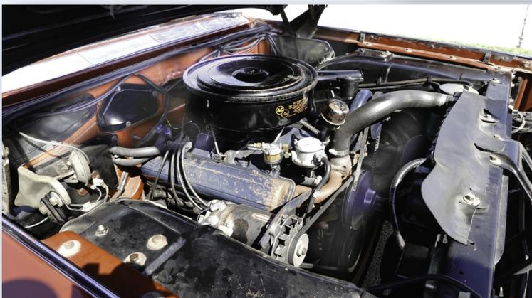
The cast iron 90 degree 6.4 liter engine is an 8 cylinder, overhead valve naturally aspirated engine with 2 valves per cylinder and a 4.0" bore and a 3.87" stroke, with a 10.5-1 compression, mounting a Carter 4bbl carburetor or Rochester 4-bbl downdraft Quadrajet. Transmission is a 4-speed Hydra-Matic (Jet-away). Neil is adding factory air.
