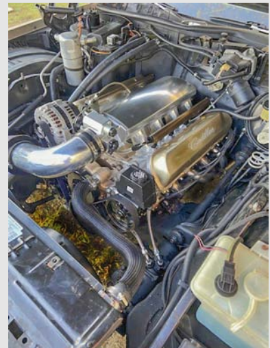
6.0L LS2 with 4160 level 2 reinforced tranny—460HP; 410hp at the rear wheels
