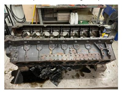
We determined the original engine block was severely damaged and a replacement block was the best path forward. Fortunately a replacement was immediately found and received within a few weeks.
